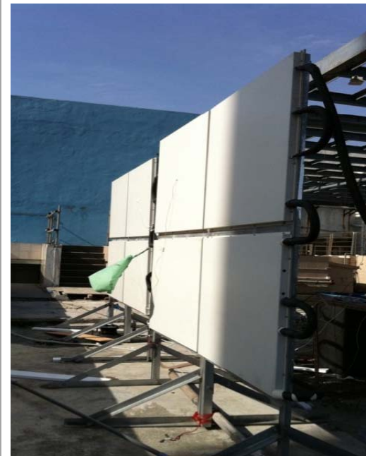
Integrated Solar Hot Water Cladding
