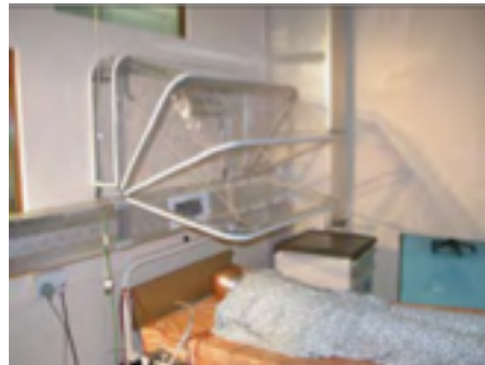
Airconditioning for SARS ward prototype
